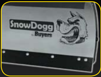
9 Moldboard tough stainless steel corrosion free moldboard
